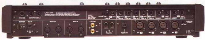
line inputs. Channels one and two also feature an additional 1/4" insert jack and channel 8 can be switched to accommodate the direct connection of an electric guitar.
