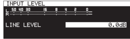
INPUT LEVEL screen when adjusting line level
